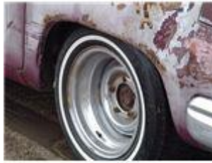
Fig.2- Rusting of Car Metal
